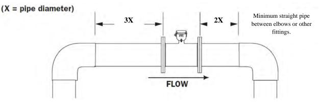
Figure C-1. Example Magnetic Flow Meter Installation.
